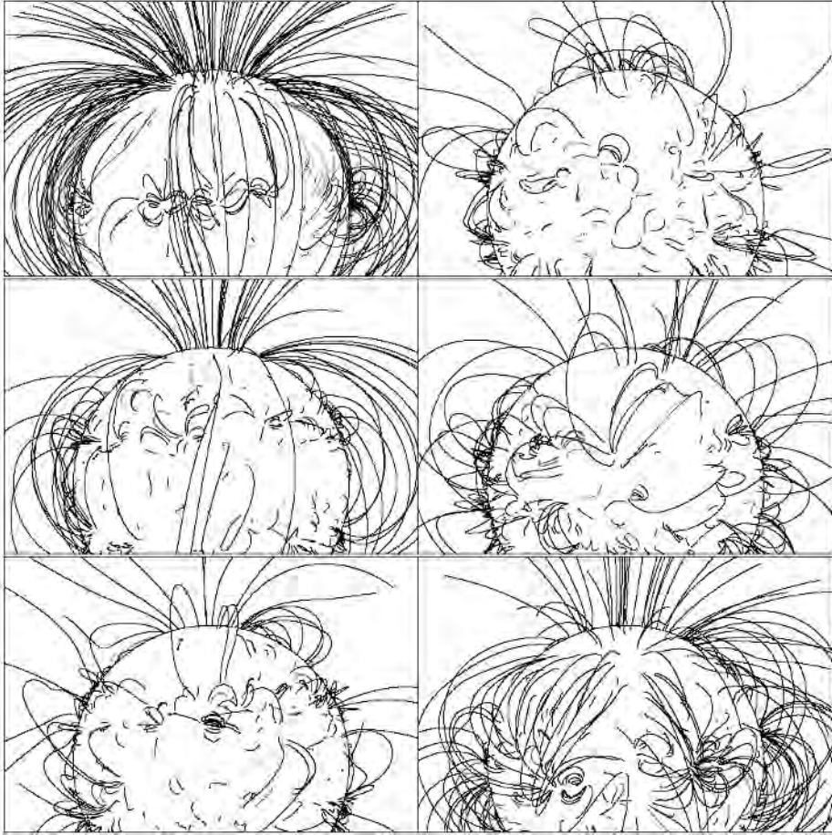
Figure 5.3: Potential field models of the global corona calculated from a source surface model during 6 different phases of the solar cycle. Each display shows 500 potential magnetic field lines, computed from simulated magnetograms that mimic the flux dispersion during the solar cycle (Schrijver & Aschwanden 2002).
